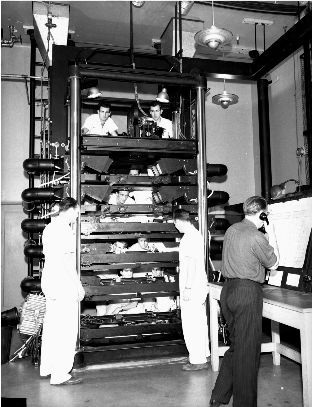
(The Disney Multiplane Camera used multiple camera operators to shoot a single scene. ©Disney.)
