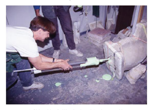
(A fabricator injects liquid latex into the Oogie Boogie puppet mold.)
