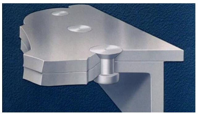
(A simple illustrated cross-section of sheet metal riveted together from FOUR METHODS OF FLUSH RIVETING)
