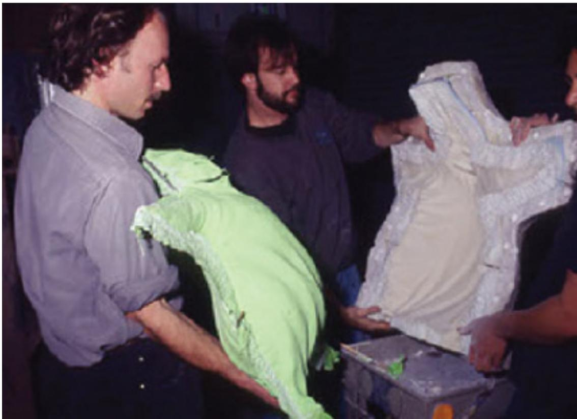
(Puppet fabricator Jon Berg removes the Oogie Boogie latex "skin" from the plaster mold after curing in a special oven. Oogie was the largest puppet fabricated for the film. )
